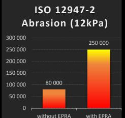
Example : Twill 2/1 98% Aramid 2% Antistatic Fibers - 225g/m<sup>2</sup>
