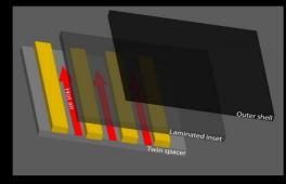
A fireman jacket lining made of TWIN SPACER® in association with an appropriate outer fabric and breathable waterproofing system provides:
